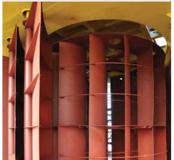
The flow control shutters and turbine rotor shaft arrangement have been manufactured and installed to the highest of tolerances, providing greater shaft torque and power outputs.
